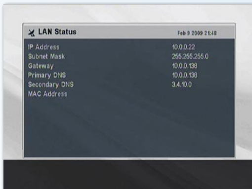
Network status displaying assigned IP addresses
