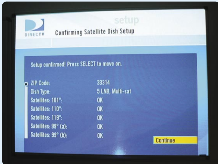
■ The DirecTV receiver's system display shows that all five satellites are being received. (99 west in Ku and Ka band)
