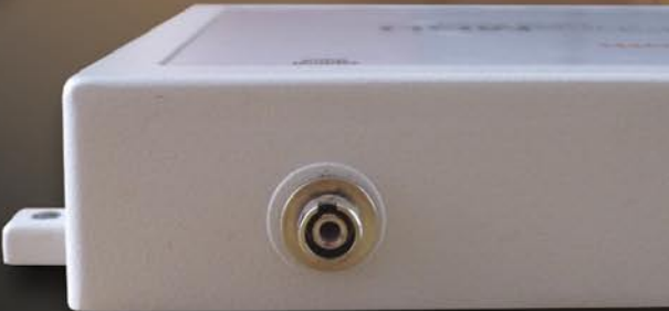
Converter Box Optical Digital Input
