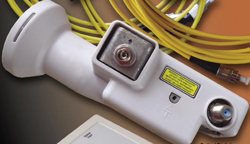
Optical Digital Output and F-Connector for the Power Supply
