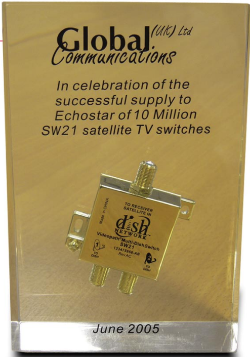
▲ One of the success products from GLOBAL COMMUNICATIONS, originally an INVACOM partner, and now melded into INVACOM: a DiSEqC switch for a US PayTV provider. 10 million of these components were produced and shipped by June 2005. It is, however, a product without much future: today DiSEqC switches are integrated in combination LNBs.
