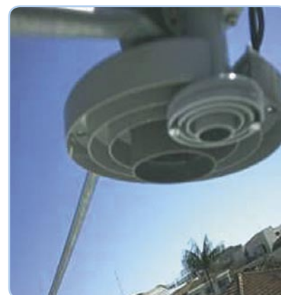
This is how simultaneous reception of C-band and Ku-band signals is achieved. Because of the prime focus antenna a grooved feed is used for the Ku-band LNB.
