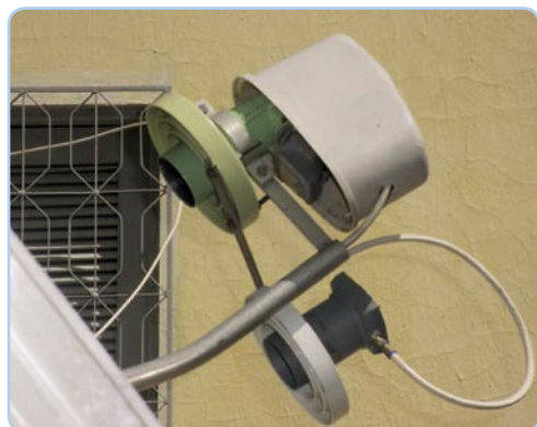
A simple solution: a metal rod connects the second feed to the focus with integrated polariser
