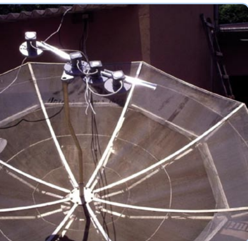
A continuous rail serves as multi-feed mount
