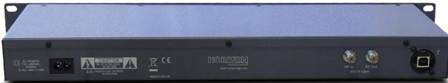
Rear panel of the transponder stream reader with a second high-speed USB interface and the antenna input. Everything else is handled by Rod Hewitt's adapted TSReader software
