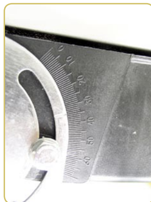
Poorly readable elevation scale
