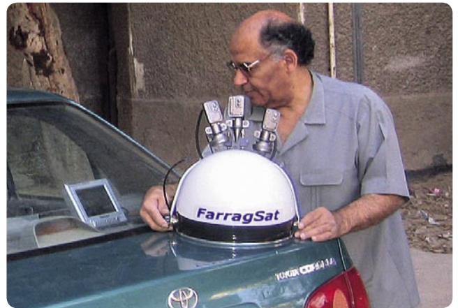
Dr. Farrag finetuning his own invention – an integral antenna. Thanks to a built-in video transmitter no cables are required for connecting the antenna to the TV set or inside a car
