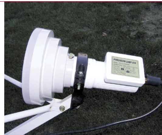
Astrotel LNBF with Cone-shaped Scalar Ring on the 1.0-Meter Dish |
