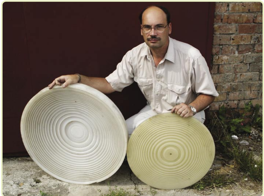
Flat (right) and paraboloidal (left) diffractive lens antennas at 35 GHz.
