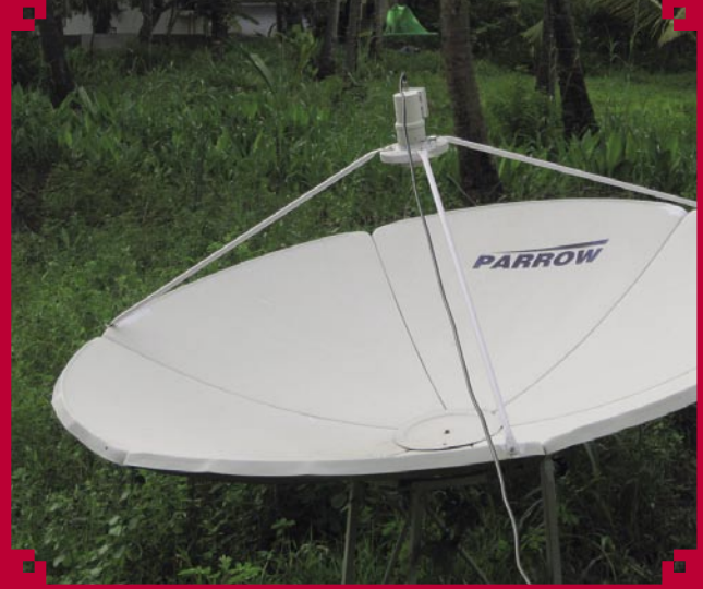
Close view of the 12-foot dish: with a little bit of improvisation it is possible to receive eight beams, namely (from above): APSTAR 6 at 134E, VINASAT 1 at 132E, JCSAT 3 at 128E, ASIASAT 4 at 122E, CHINASAT 6B at 115.E (this LNB is the one that is in focus), NSS 11 at 108 in the Ku-Band, ASIASAT 3S at 105.5E und ASIASAT 2 at 100.5E
