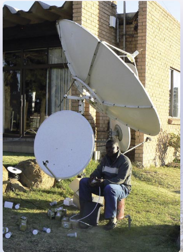
Functionality test for newly arrived LNBs: a technician tests every LNB by connecting it with a signal analyzer and then by attaching it to a dish pointed at 68.5° east.
