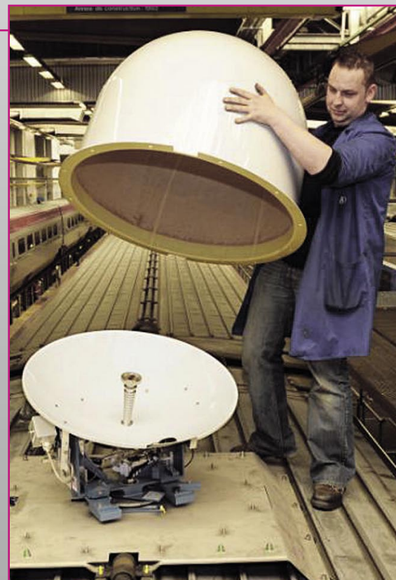
Finished! The radom is placed on top of the antenna. Now the system is not only protected from the weather but also from the enormous 300 kph (188 MPH) wind load.
