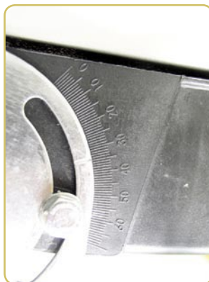
Poorly readable elevation scale
