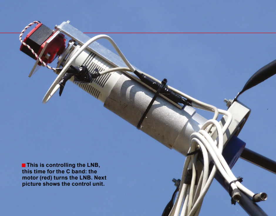
■ C band reception with only a small antenna? No problem, if you know how and where to mount the LNB. One antenna manufacturer has equipped a 1.2m dish with alternative rods that allows to arrange both the Ku band LNB in the focal point and the C band LNB outside the focal point using a rail system. Even the DiSeqC switch fits in. "At our location this system allows reception of three C band satellites at 40° East, 5° West and 30.5° East," explains Berndt Rosenberger.
