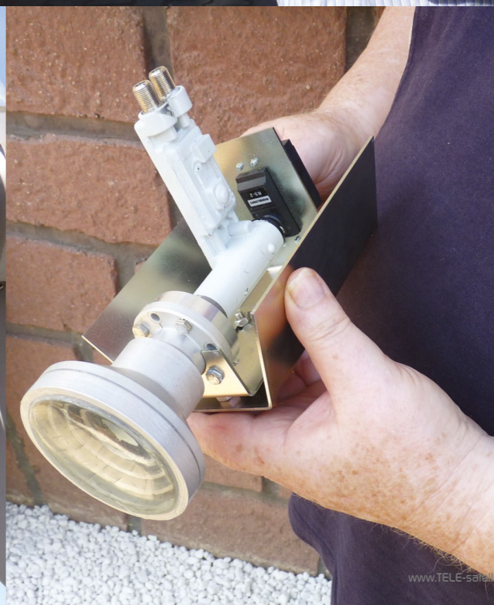
■ Another invention: Thanks to a small motor the Ku band LNB can be skewed. On the second picture you can see the component before installation, and the third picture shows the control unit.
