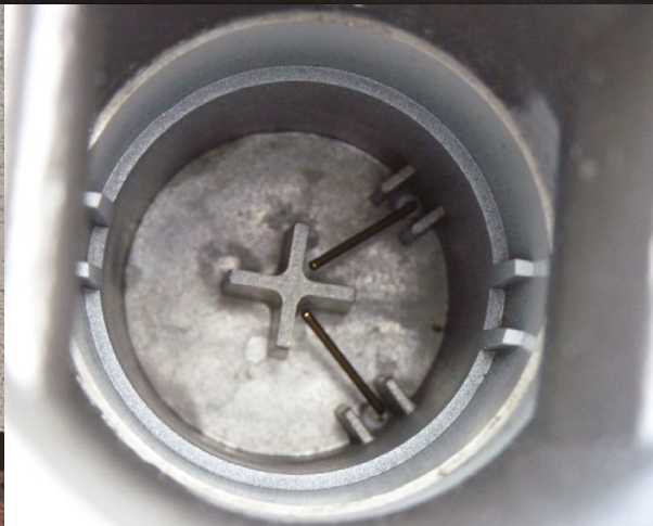
■ A look inside the AVCOM LNB: Only the cross-shaped element in the background is rotated. Depending on the 45° turn either linear or circular signals can be received.
