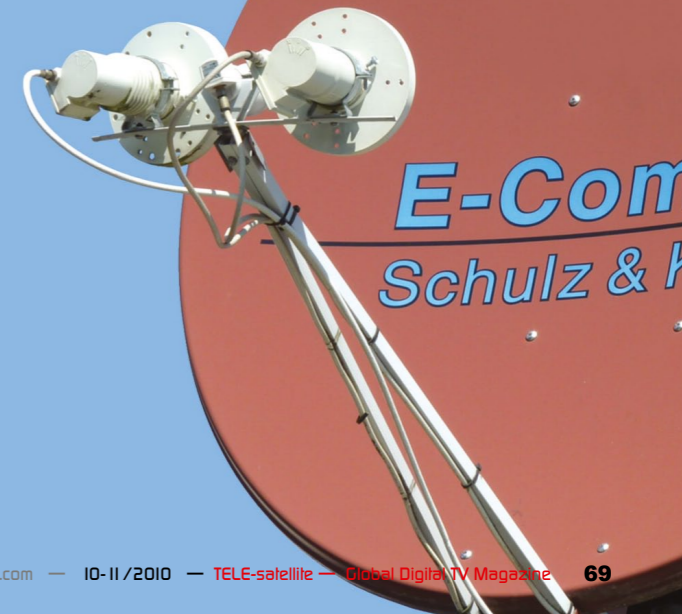
■ Another invention: Thanks to a small motor the Ku band LNB can be skewed. On the second picture you can see the component before installation, and the third picture shows the control unit.
