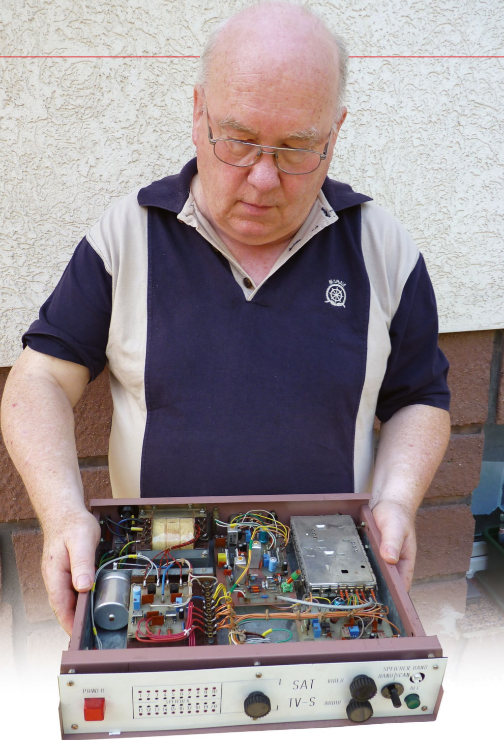
■ How it all began: Rainer Schulz's first self-made receiver dating back to 1988. He sourced individual components such as the tuner and a chipset from West Germany, but all the rest is 'proudly made in the GDR'.
