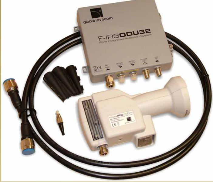
The complete Outdoor installation kit with the new FIRS LNB and the standard cable exactly 1.5 meters in length with "N" connectors on both ends to provide an optimal connection between the F-IRS LNB and the F-IRS ODU32. Longer cable lengths are not recommended since the signal attenuation in the upper frequency ranges (up to 5.45 GHz) is much too high. Global Invacom has matched its system precisely to this specific cable.
