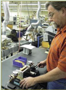
Bill Adamo is Quality Control Group Leader and shows us how the weather-tight seal of a filter is pressure tested: "The filter is placed here and pressurized with air at 5 PSI."
