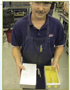
■ Dale Newton shows us the production sequence: out of a solid block of aluminum (left) a complete filter body is milled with all the openings for connectors and screws (right).
