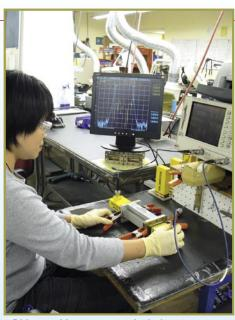
■ Did everything run correctly during production? Thuy Naylor performs a final test to determine if the filter lives up to it's specifications by connecting it to a network analyzer to confirm performance.
