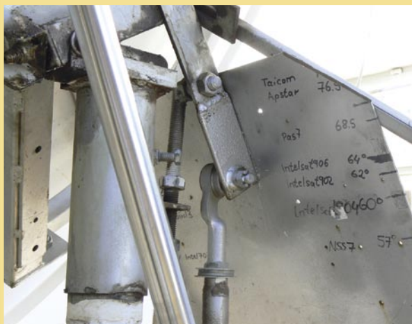
Absolutely essential while turning the antenna is a positioning guide such ▲ as this metal plate with numerous position notations.
