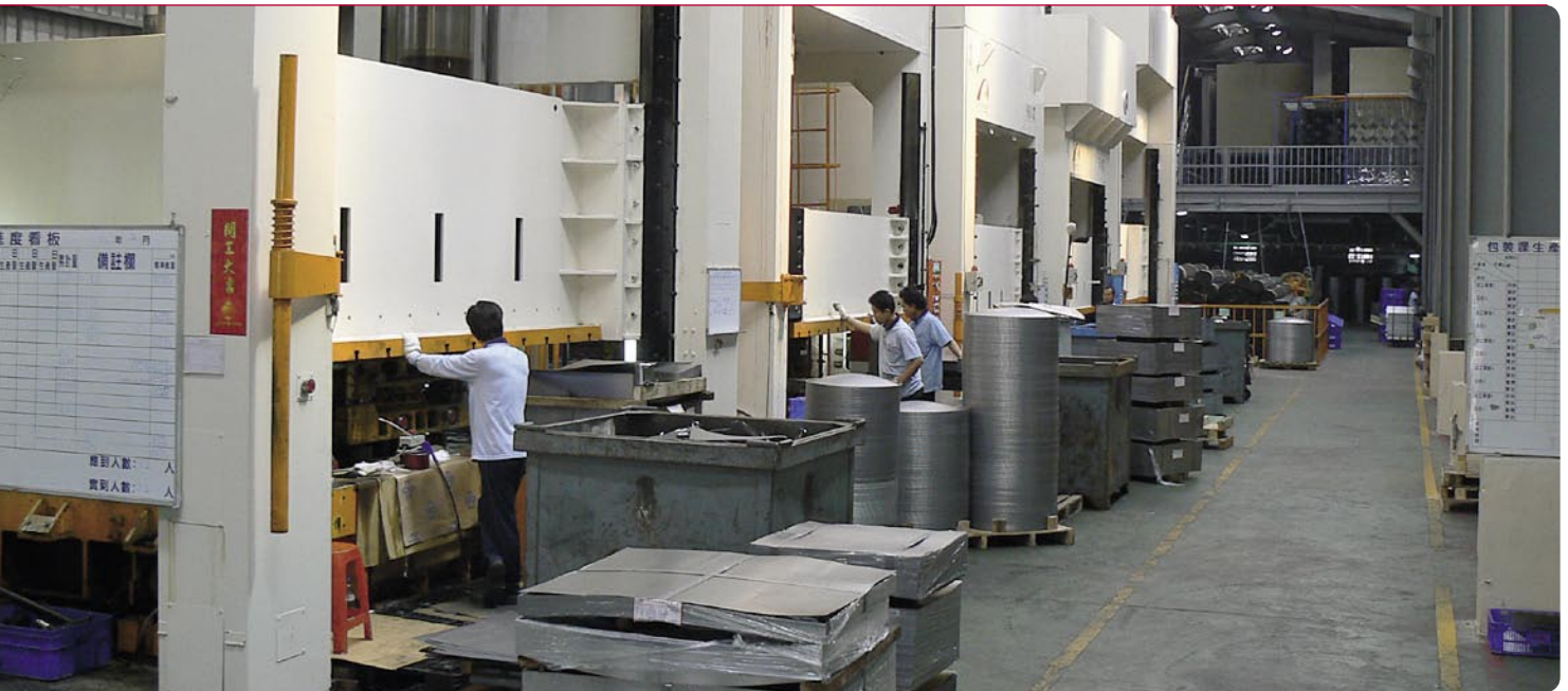
The pressing machine: the precut sheet metal (on the pallet in the foreground) is placed flat in the pressing machine and comes back out as an offset antenna.
